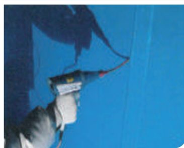
PE Weld Zone Spark Test (Leak inspection)
